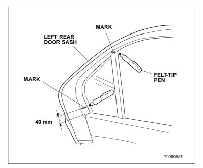
7. Temporarily position the two frame clips on the door sash aligning the end of the frame clips with the marks you made in step 4 and attach the pieces of masking tape as shown.
